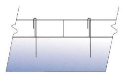
Cross section of installed Erocell
