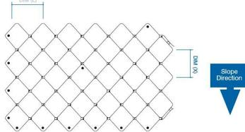
Plan View of Installed Erocell DIM (L) = 10m (Panel Length) DIM (X) = 7m (Panel Width)
